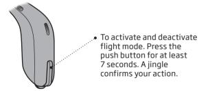
Opening and closing the battery drawer will also deactivate the flight mode. See section: Quick reset.
